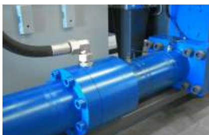
Strong pressing operation by amply dimensioned cylinder
